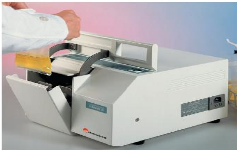
Figure 36.10 A stomacher. Paddles in this specialized blender homogenize the solid food sample in a sealed, sterile bag. The sample is suspended in a sterile solution.
