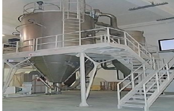
Figure 36.1 Spray dryer. Industrial spray dryers are used to dry or concentrate large volumes of high-value liquid foods.
